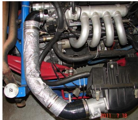
Optional heat shield sock installed
