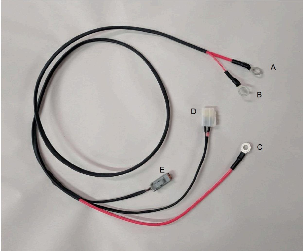
Install the updated harness along the diagonal round chassis tube, then the vertical round chassis tube. Next attach the harness to the bottom of the 1" longitudinal square tube, above the fuel cell enclosure. Take care to keep the harness off the edge of the fuel cell enclosure. Then route the harness across to the master switch, secure with ty-wraps as necessary.
