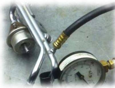
2. Remove the vacuum reference line or hose from the Stock Regulator. Start the car briefly to take a fuel pressure reading, record for the starting point of the adjustable regulator.
