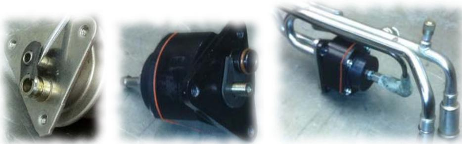
*Note: it's very helpful to use some sort of lubricant. Like WD 40 Carefully to install the New Regulator onto the fuel rail.*
