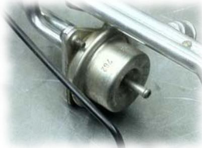
3. Remove the Stock Regulator: First bleed the residual fuel pressure from the system. Carefully remove the fasteners from the regulator.
